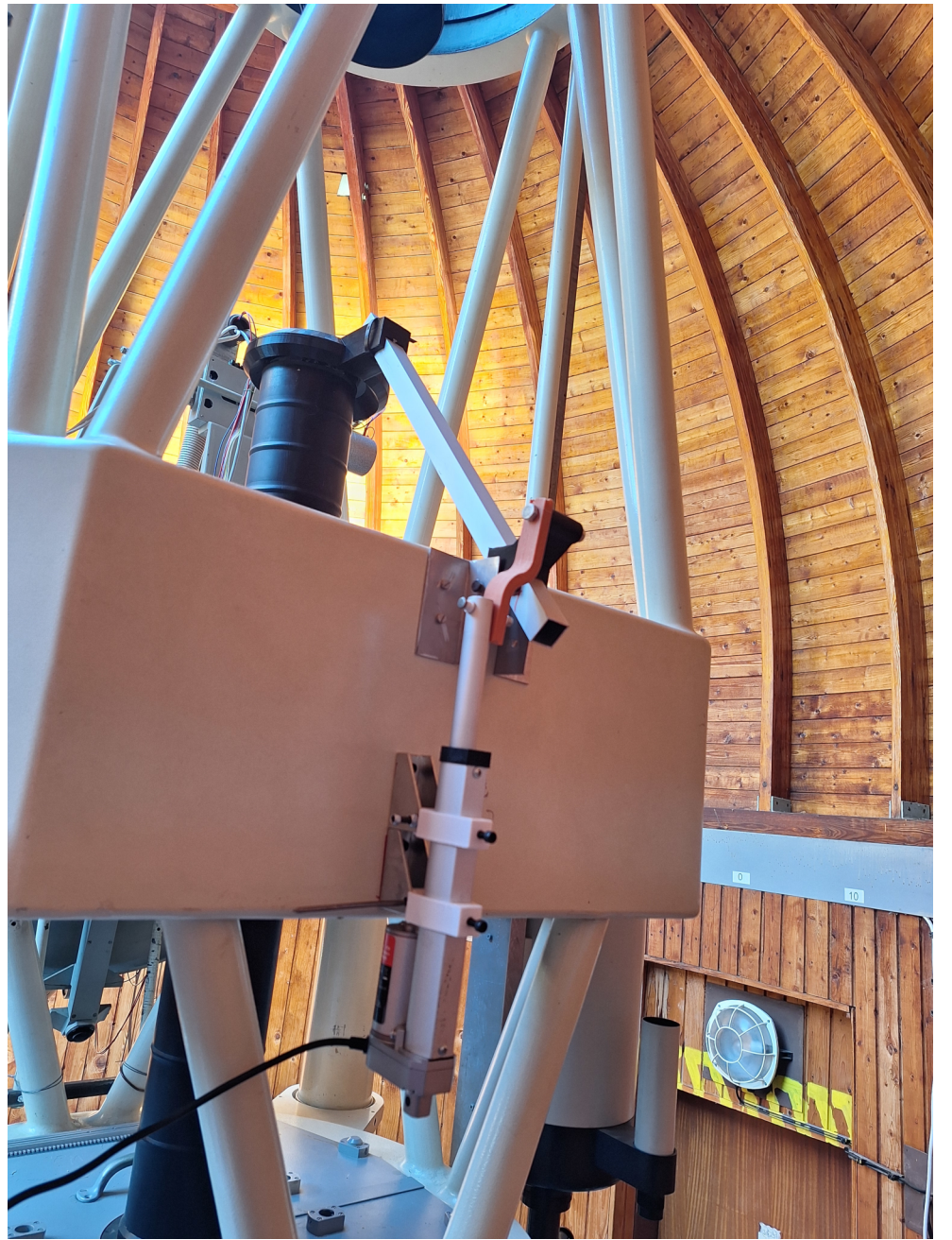
Linear actuators, scrapy aluminium extrusions and some 3D printed parts
