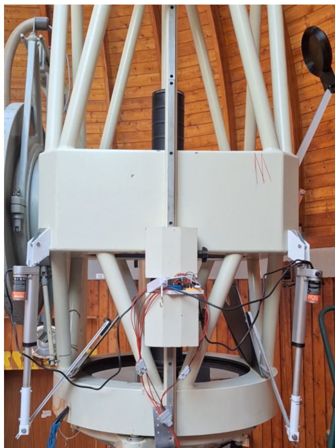
Telescope unpacking - Opening covers by 3 linear actuators, scrapy aluminium extrusions and some 3D printed mechanical connecting parts. Controlled by 6 relays and 6 digital outputs
