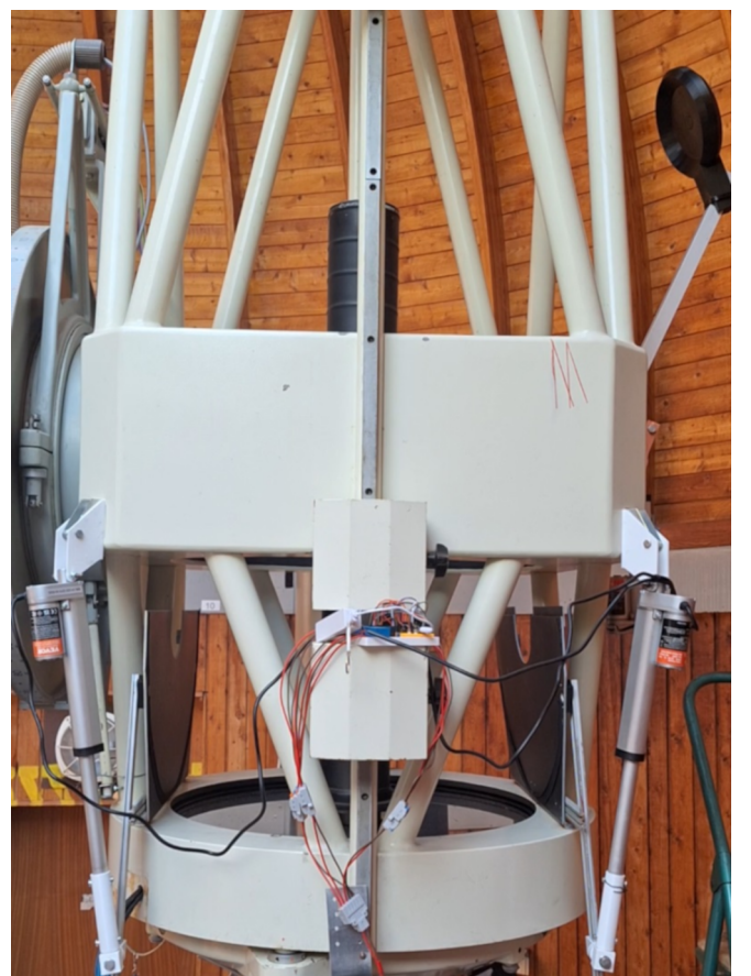
Telescope unpacking - Opening covers by 3 linear actuators, scrapy aluminium extrusions and some 3D printed mechanical connecting parts. Controlled by 6 relays and 6 digital outputs
