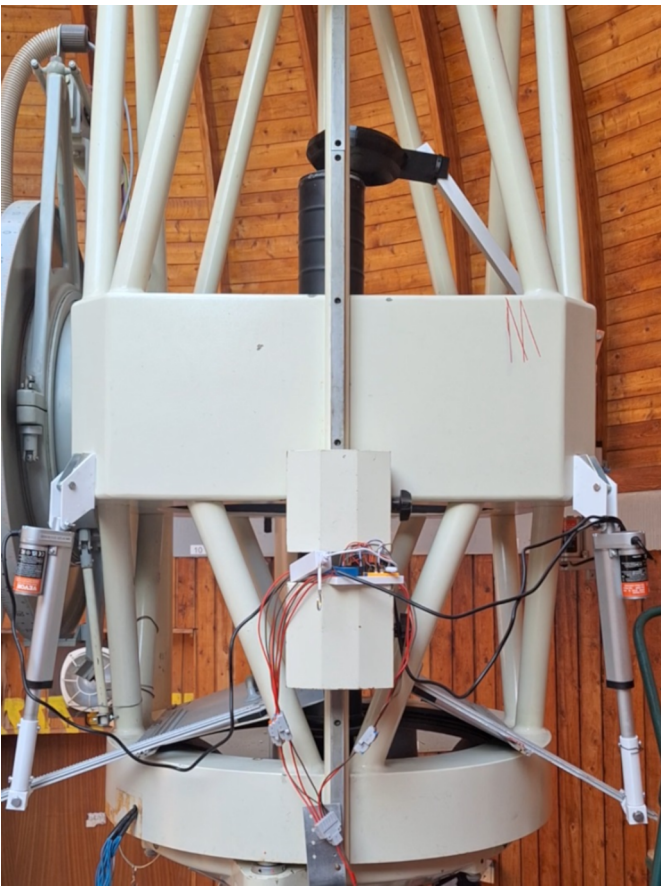
Telescope unpacking - Opening covers by 3 linear actuators, scrapy aluminium extrusions and some 3D printed mechanical connecting parts. Controlled by 6 relays and 6 digital outputs
