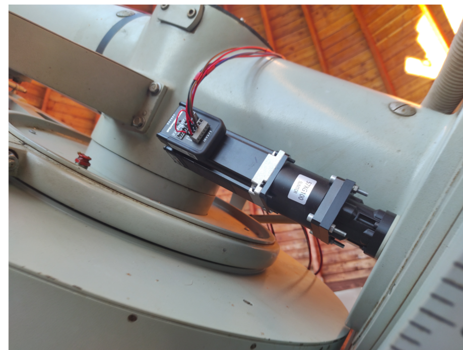
Detail of NEMA23 motor with installed gearbox reducer and 3D adapter to internal gearing output at RA/HA axis for fine movements
