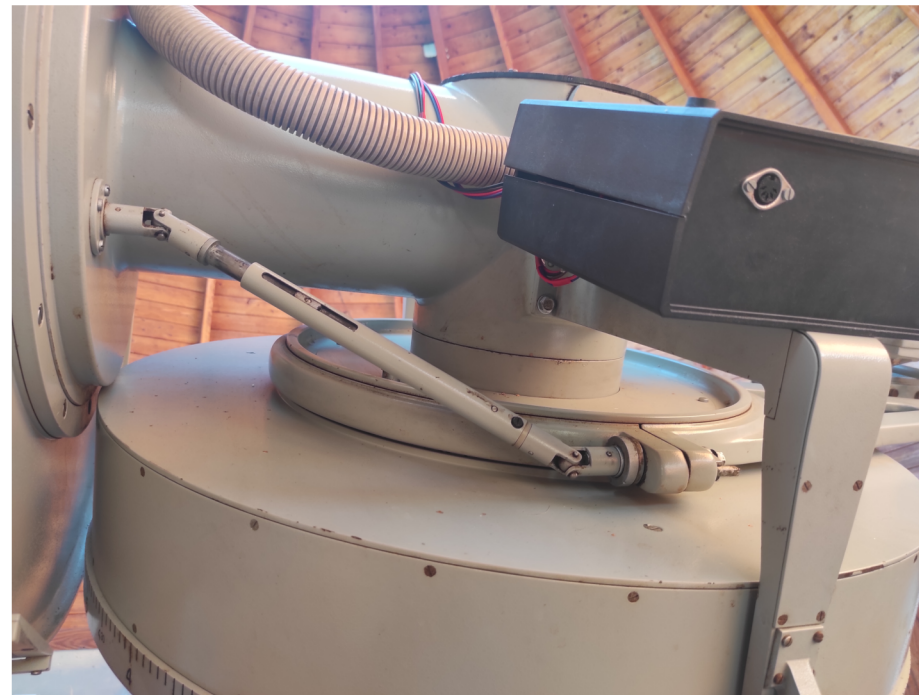
Detail of internal gearing output at RA/HA axis - locking off RA/HA axis - replaced with NEMA23 motor with installed gearbox reducer and 3D adapter (out of second picture - cables visible) with 3D printed knob for locking of RA/HA axis
