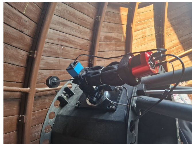
Fig. – Final installation of spectrograph on AGO70 performed in August 2024.
