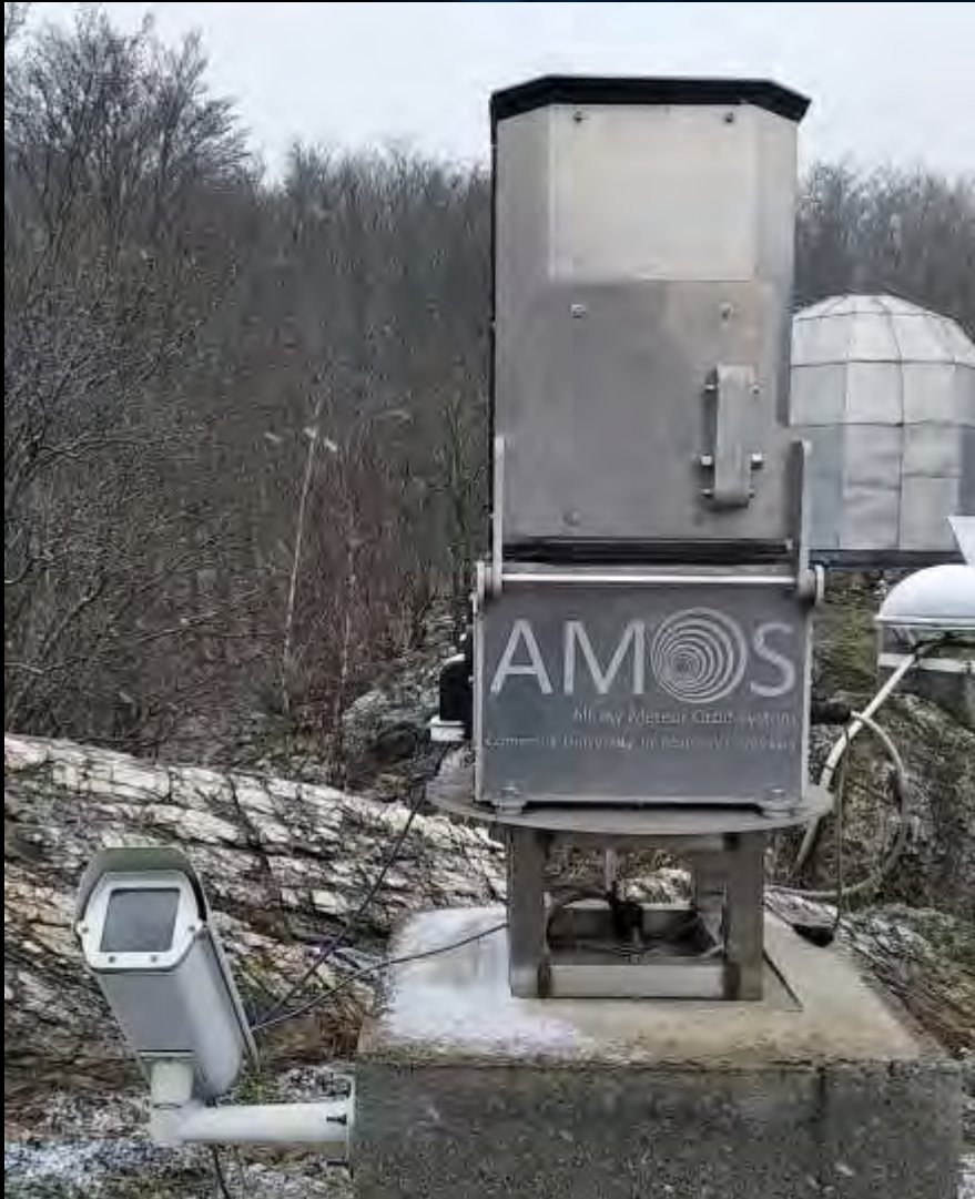
Fig. 15. The All-sky Meteor Orbit System (AMOS) camera
