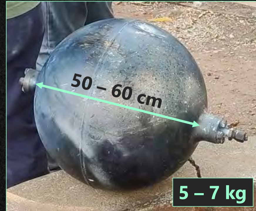
Figure: Hydrazine tank from re-entry of CZ-3B. Source: universemagazine.com
