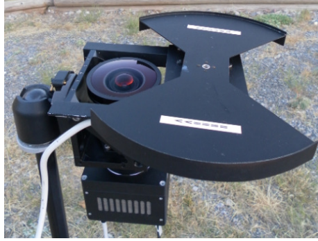
Figure 1. A SPOSH camera with a rotating shutter
