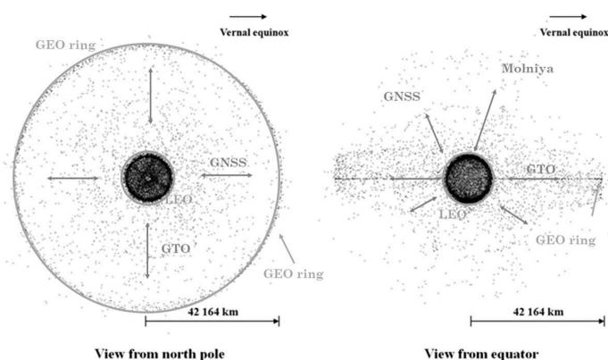
**Figure 1.** Space debris spatial distribution. Data generated by the using public catalogue [www.space-track.org](http://www.space-track.org) (Šilha , 2012).
