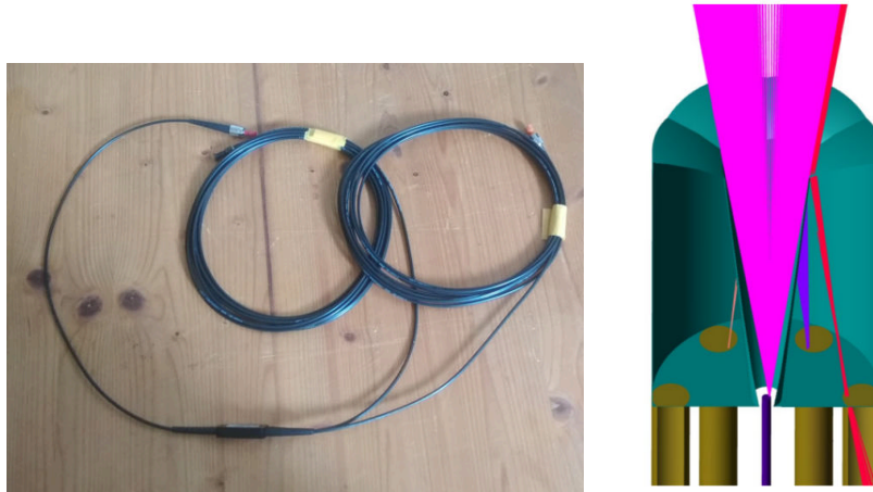
Figure 2. Example images of the tip-tilt sensor system : Left) The camera image of the fibre bundle. The end on the left hand side contains seven fibres, a single mode central core and six larger sensing cores. These are split off into two bundles (terminating on the right), one with a sole single mode core and the other with six larger cores for sensing. Right) The preliminary microlens design, adapted from Hottinger et al. (2018).
