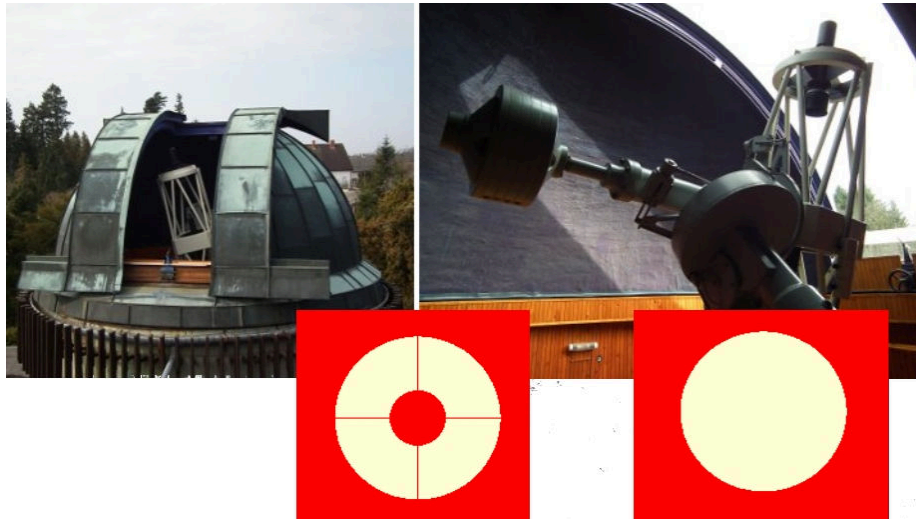
Figure 1. The 600/7500 Zeiss telescope of the Gothard Observatory, a typical Cassegrain instrument. The left inset shows the shape of the aperture, occulted by the secondary mirror and its holders, while the unocculted aperture of the same size is shown by the right one.
