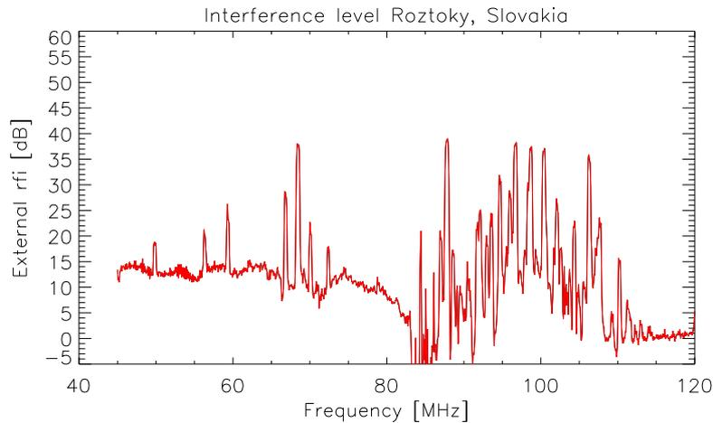
**Figure 3.** A spectral overview with 1280 channels from a log-periodic broadband antenna measured at the Roztoky observing station. A relatively low interference level below the FM-band indicates, that the system is suitable for solar burst observations at those lower frequencies. The frequencies 70.45 - 74.8 MHz are reserved for radio astronomy but shared with other mobile services.
