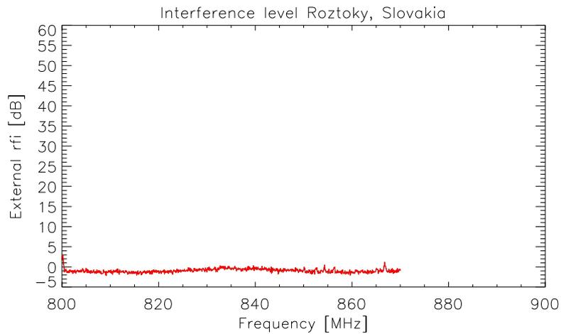
**Figure 11.** A spectral overview with 1120 channels measured at the Roztoky observing station. A very low interference level in this whole sub-band makes the latter suitable for solar observations.
