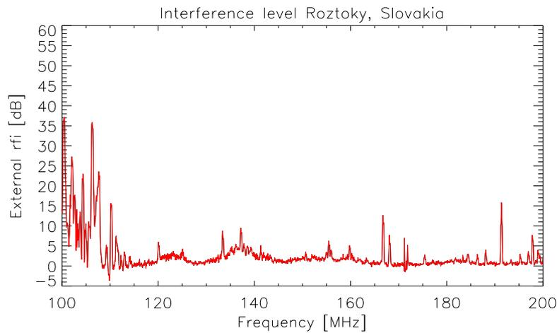
**Figure 4.** A spectral overview with 1600 channels measured at the Roztoky observing station. Relatively low interference levels between the FM-band and VHF indicate, that the system is suitable for solar observations in that range. The frequencies 150.4 - 151.4 MHz are reserved for radio astronomy, but shared with other services.
