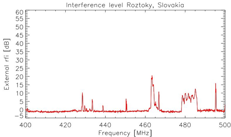
**Figure 7.** A spectral overview with 1600 channels measured at the Roztoky observing station. The rather low interference level is perfect for solar observations below 460 MHz. The frequencies 406.1 - 410 MHz are reserved for radio astronomy (solar flux monitoring), but shared with other services.
