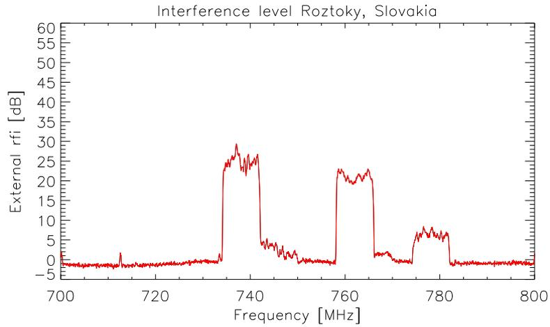
**Figure 10.** A spectral overview with 1600 channels measured at the Roztoky observing station. A very low interference level can be seen in this band. This range would be ideal for solar observations of decimetric pulsations. However, there are two strong DVB-T channels which reduce the number of RFI-free channels.
