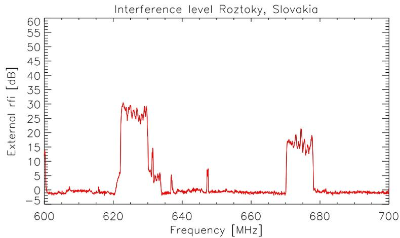
**Figure 9.** A spectral overview with 1600 channels measured at the Rostoky observing station. A rather high interference level can be seen in this band. The frequencies 608 - 614 MHz are reserved for radio astronomy (solar flux monitoring and pulsar observations), but shared with other services. Above 620 MHz there is a strong DVB-T interference, but some individual channels may be used for solar observations.
