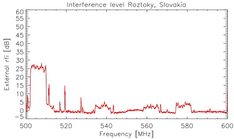
**Figure 8.** A spectral overview with 1600 channels measured at the Rostoky observing station. A high interference level can be seen in this range. The channels are used for DVB-T.
