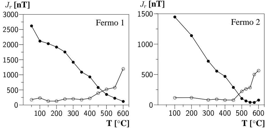
**Figure 2.** Thellier method, demagnetization (*full circles*) and magnetization (*open circles*) curves of both Fermo 1 and Fermo 2 samples. ( $J_r$  - remanent magnetization in nano Tesla (nT) with respect to temperature T).
