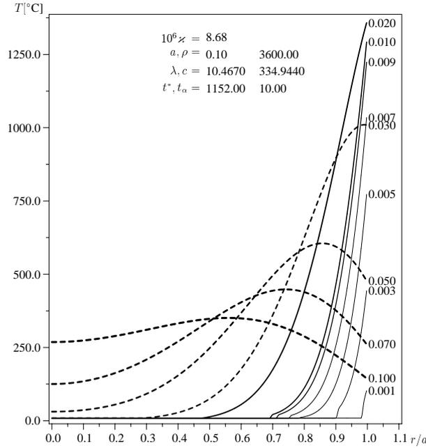
**Figure 5.** Radial distribution of the temperature inside the sphere for various times. The numeration of curves denotes  $(t/t_* = t\zeta/a^2)$ .
