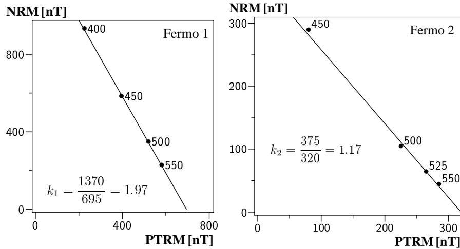
**Figure 3.** Graphical illustration of data NRM/PTRM for computation of coefficients  $k_1$  (Fermo 1),  $k_2$  (Fermo 2). NRM – natural remanent magnetization; PTRM – partial thermoremanent magnetization of the samples.
