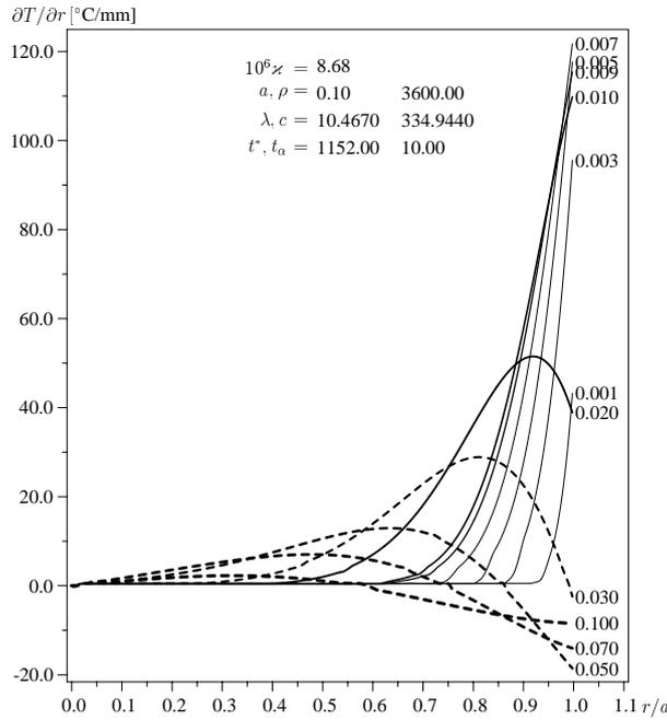
**Figure 6.** Radial distribution of the temperature gradient inside the sphere for various times. The numeration of curves denotes  $(t/t^* = t\pi/a^2)$ .
