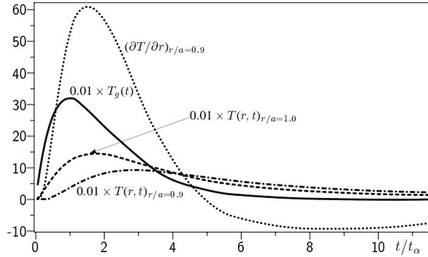
**Figure 7.** Time evolution of the temperature (multiplied by factor 0.01) of the hot gas  $T_g(t)$  – full line, surface temperature of the sphere  $T(r, t)$  for  $r = a$  – dashed line, temperature at radius  $r = 0.9 \times a$  – dash dotted line. The dotted line is time course of the temperature gradient (in  $^{\circ}\text{C}/\text{mm}$ ) at radius  $r = 0.9 \times a$ .
