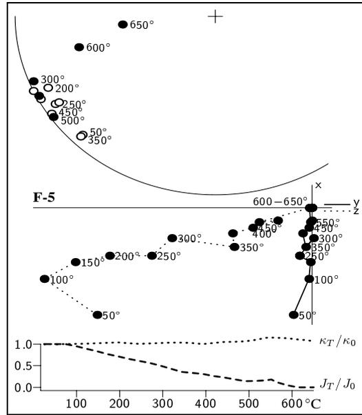
**Figure 1.** Thermal demagnetization of sample F-5, stepwise heating to 650°C; Zijderveld diagrams and stereographic projection of the remanent magnetization (RM); *full circles* - positive, *open circles* - negative RM (in stereographic projection);  $\kappa_T$ ,  $\kappa_0$  – magnetic susceptibility at T and at 25°C, respectively;  $J_T$ ,  $J_0$  – remanent magnetization at T and at 25°C, respectively.
