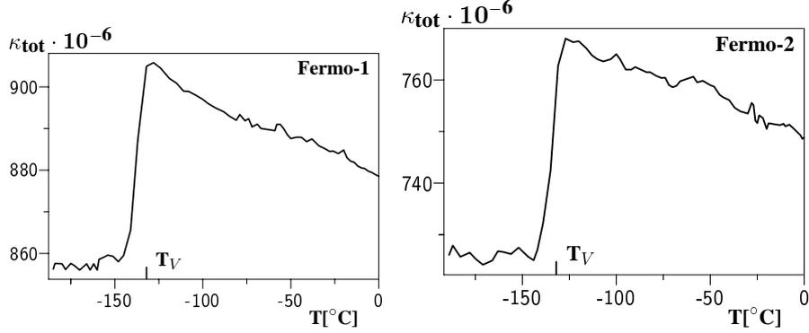
**Figure 4.** The detection of the Verwey transition temperature ( $T_V$ ) of nonstoichiometric magnetite in Fermo samples. The measurements of the change of magnetic susceptibility ( $\kappa$ ) of samples within the  $0^\circ\text{C}$  and  $-190^\circ\text{C}$ .
