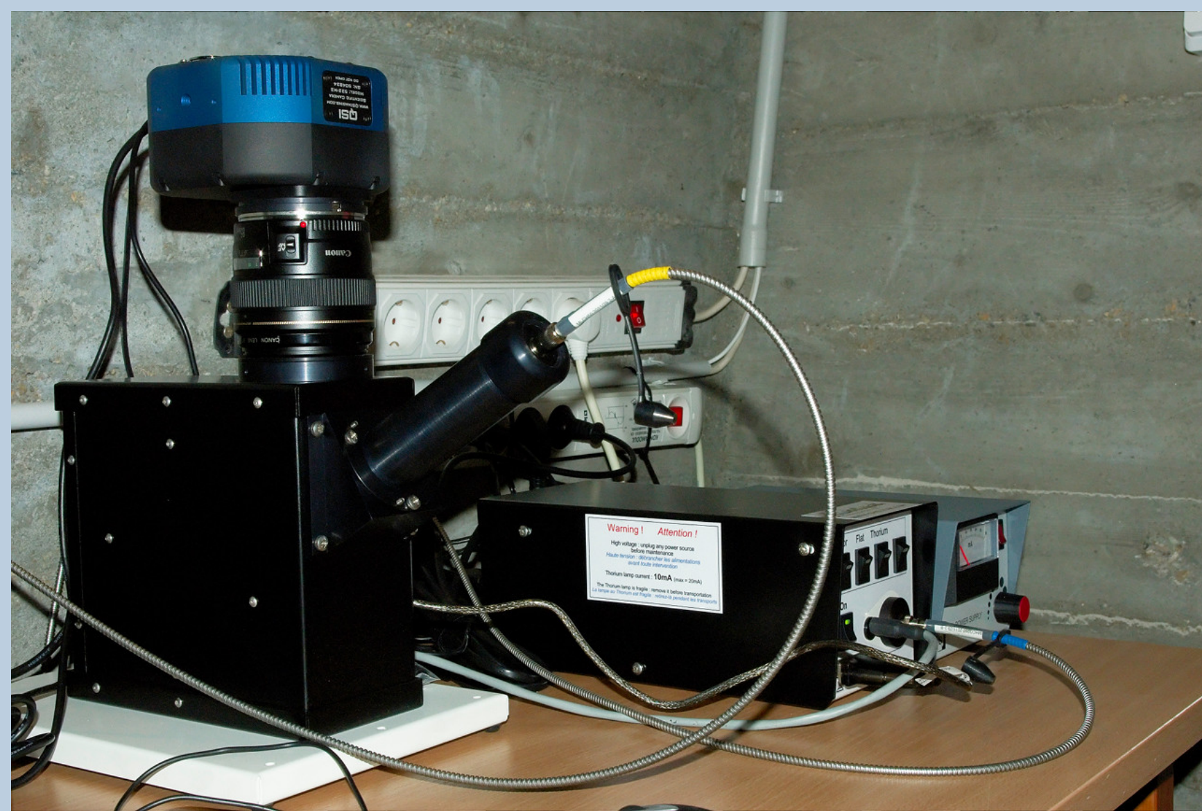
The eShel echelle spectrograph and its accessories: QSI 532ws CCD camera and the ThAr unit with its power supply box in a thermally isolated concrete room below the 0.5m RC telescope of the Gothard Astrophysical Observatory.
