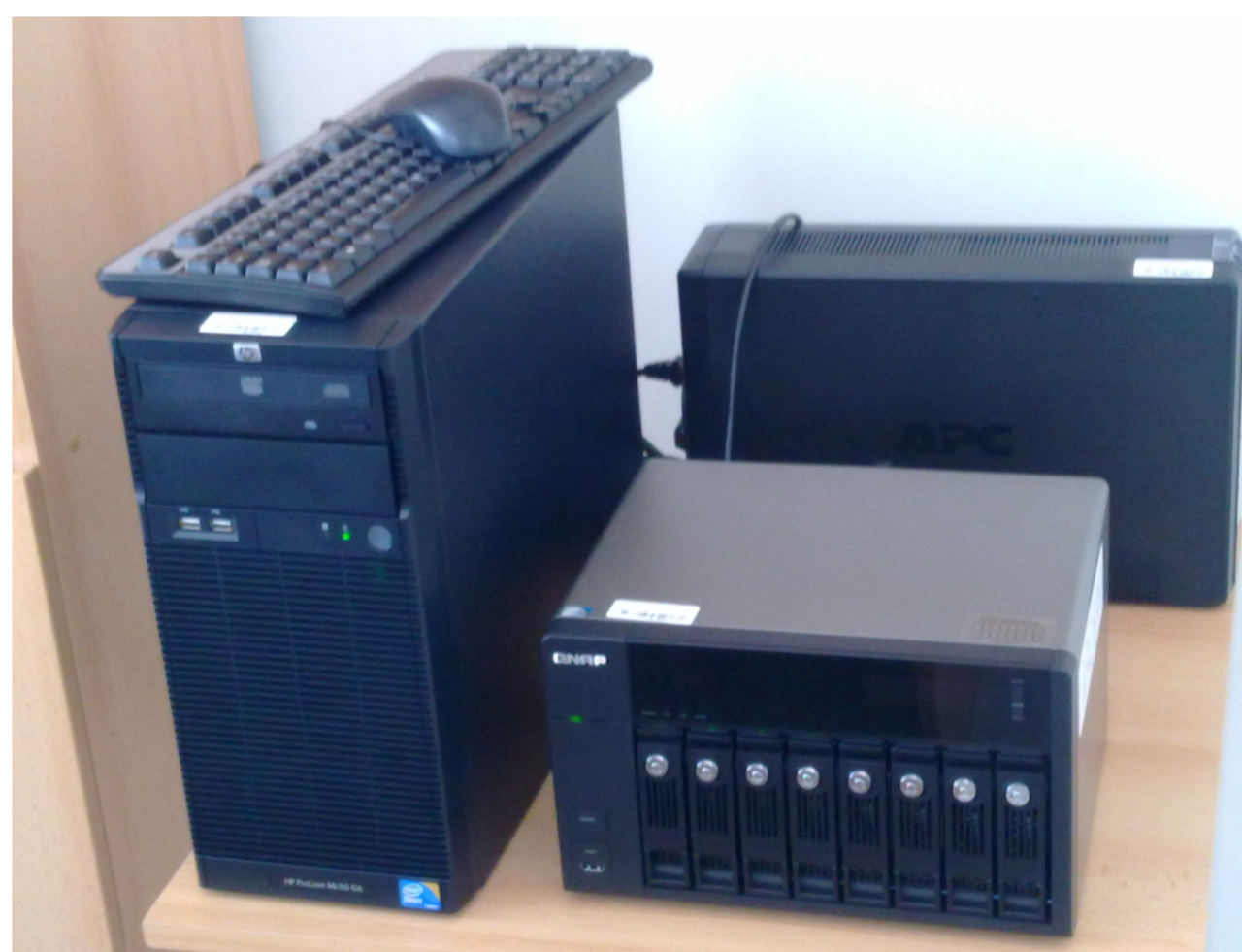
Fig. 1. Server and RAID-6 disk array used for MUNI Photometric Archive
