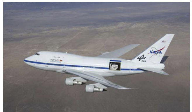
Fig. 41. Photo of SOFIA, the Stratospheric Observatory for Infrared Astronomy, during 'open-door' flight tests.
